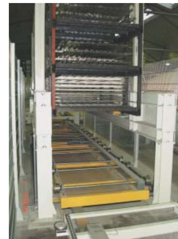
Vollkorbstapler zur Bildung von Ofenbatches Full rack stacker for the formation of a furnace batch
