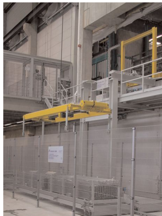
Korbtransport ins Obergeschoss Rack transport to the upper storey
