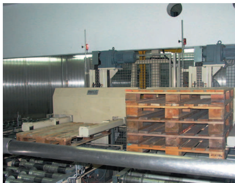
Stacking devices for narrow and for wide wooden pallets on the platform in the upper level
