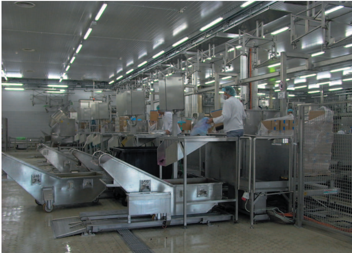
Consignment workplaces on the upper level; behind them is a transverse transport trolley for the storage units
