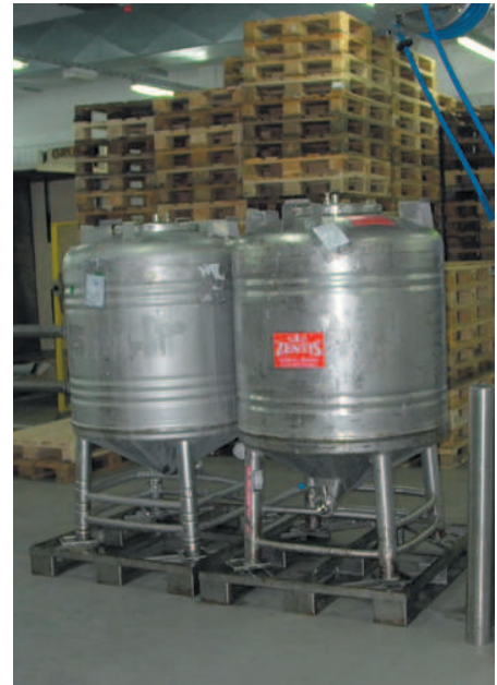
Zentis containers are stored on special auxiliary pallets. Only approved load carriers are used and that the goods are stored in a stable manner.
