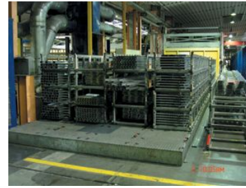
Section racks behind the ageing furnace for press P2
