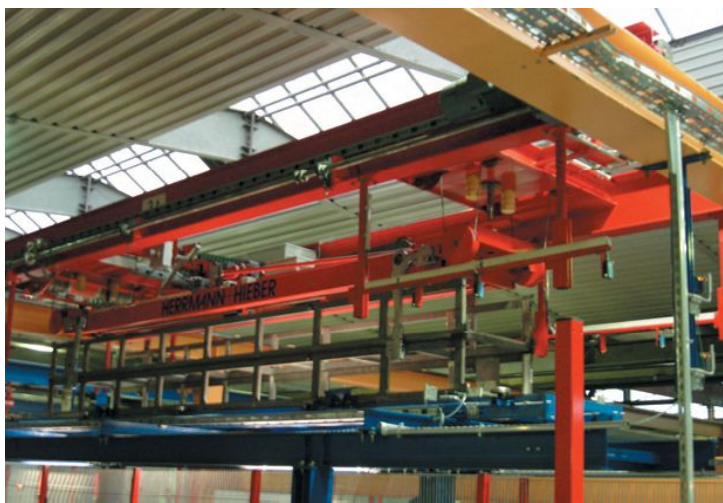
Automatic crane AMK 2.2 with a double gripper for the simultaneous transport of two section racks
