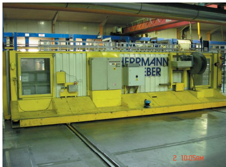
Transport trolley that can move transversely to the blow-clear station for sections up to 8,100 mm long
